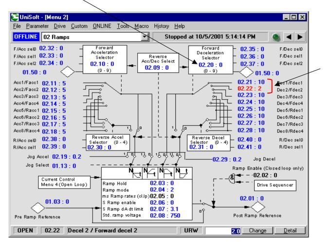
Since there are 8 decel rates, 3 control lines could select any one of 8. If we investigate the properties of the Decel Reference Selector #2.20 we find a truth table describing which decel rate is selected per each of the 3 controlling inputs (bits) to the #2.20 selector.
